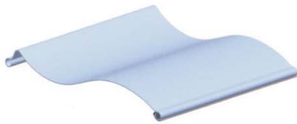
Model AR92-S with S-shaped aluminium louver - Louver width 92 mm, - Louver thickness 0.44 mm
